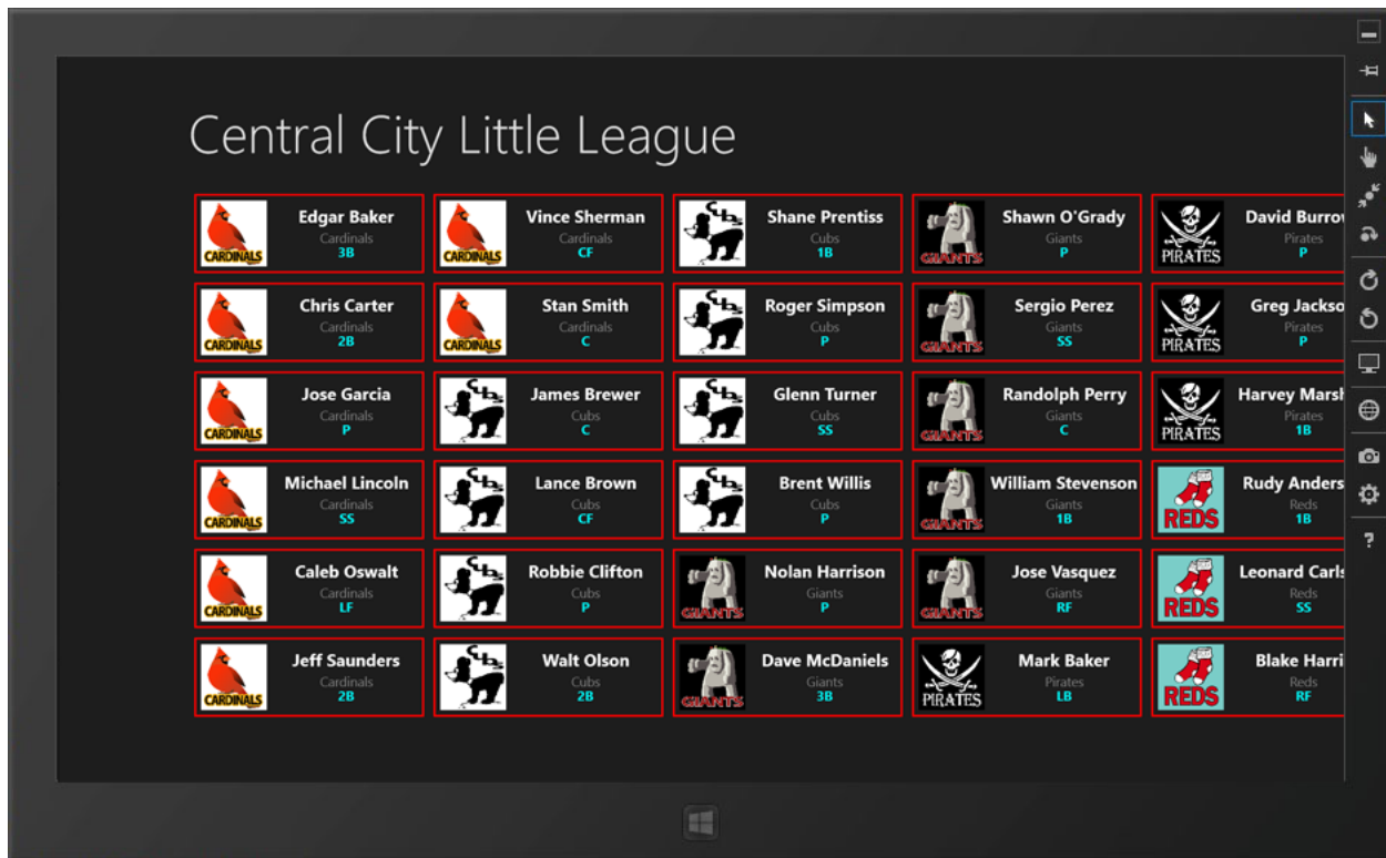
Figure 16 – Multiple fields can be concatenated to produce primary, secondary, and tertiary sorts. In this example, the data is sorted primarily by team, secondarily by the player's last name, and thirdly by the first name.
