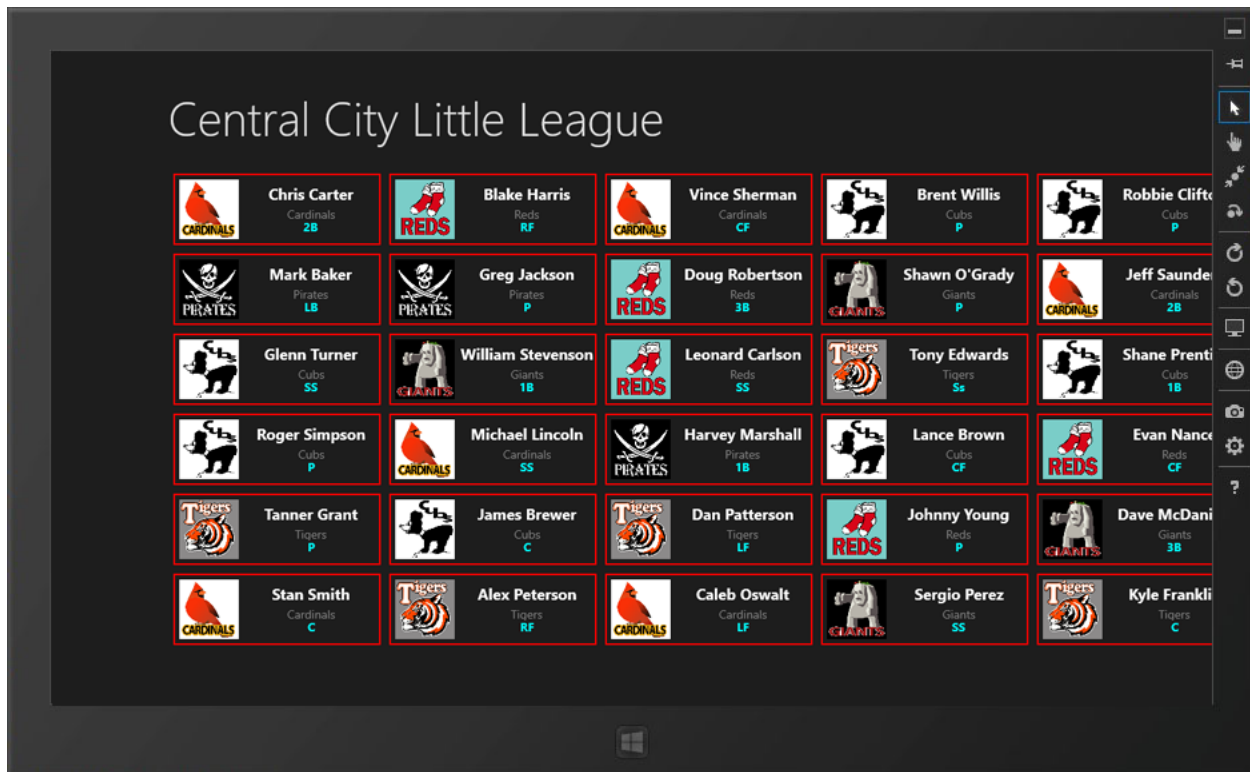
Figure 12 – The GridView displays data in a series of columns and can be scrolled horizontally to view more data if necessary.
